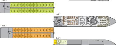
SHIPYARD: Neptun Werft GmbH, Warnemünde PASSENGERS: max. 174 guests | CABINS: 86 outside cabins per ship FLAG: Germany | LENGTH: 125.8 m | WIDTH: 11.4 m SPEED: max. 24 km/h | POWER: 2 × 800 kW/a total of 2,174 HP YEAR OF CONSTRUCTION: 2005 A-ROSA STELLA
